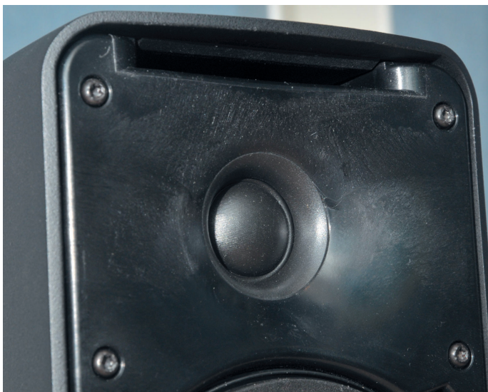
Tweeter with waveguide integrated into the frontal plate to control directivity and to boost the sensitivity of the tweeter.
