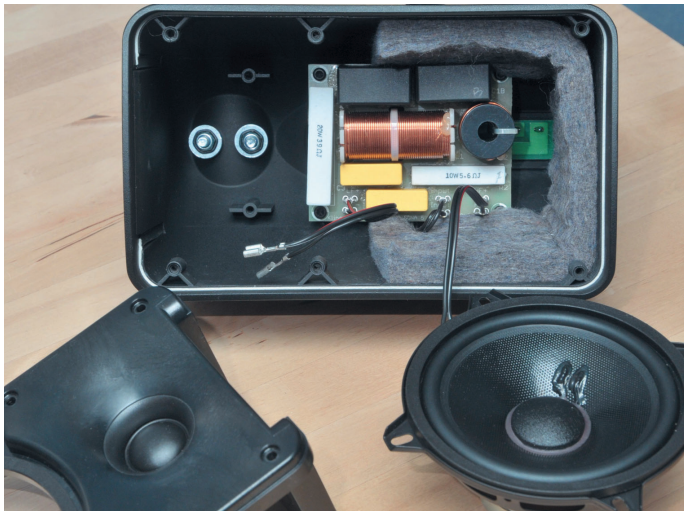
A Sona 5 taken apart: the enclosure is made of the frontal plate and the actual shell. Both are made from flame-protected plastic.
